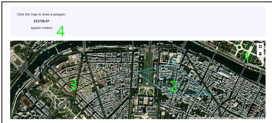
Figure 1: The IPOL's map interface. 1) The controls to draw and remove polygons, 2) A polygon already draw, 3) A polygon being drawn, and 4) the information about the current polygon.
