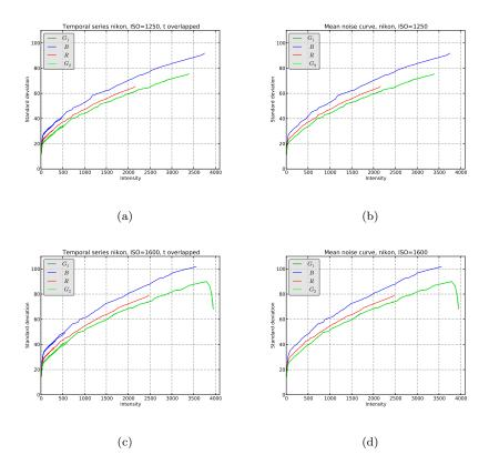
FIGURE 1. Noise ground-truth curves obtained for a Nikon D80 camera with fixed ISOs of 1250 (a) and 1600 (c) and four exposure times,  $t \in \{1/30s, 1/250s, 1/400s, 1/640s\}$  using laboratory calibration. Channels  $G_1$  and  $G_2$  give the same STD. The obtained curves overlap perfectly. Since they cover different color intervals, their fusion yields a complete noise curve (b), (d).
