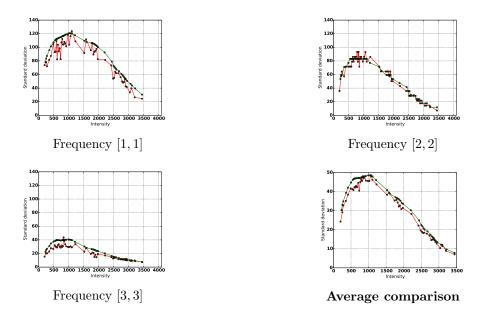
FIGURE 7. Comparison of the temporal (ground-truth, in green) and spatial STD (in red) for the Canon EOS 30D in JPEG-encoded images with quality factor Q = 92 for ISO speed 1600 using blocks of  $4 \times 4$  DCT coefficients. The curve at the bottom right is the comparison between the averaged temporal STDs and the averaged mean spatial STDs (along all frequencies except DC), showing that in average both estimations match.
