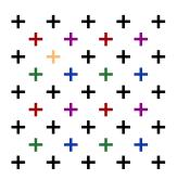
FIGURE 5. Position of the center of pixels in the original image  $\tilde{u}$  in black, in the four sub-images  $\tilde{u}_1$  in red,  $\tilde{u}_2$  in purple,  $\tilde{u}_3$  in green and  $\tilde{u}_4$  in blue. The yellow pixel will be reconstructed by averaging the top left red pixel, the top right purple pixel, the bottom left green pixel and the bottom right blue pixel of its four pixel neighborhood.
