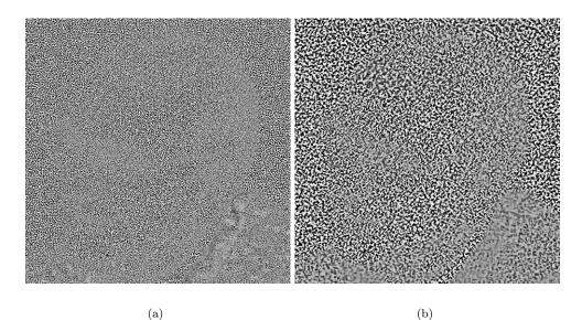
FIGURE 6. Detail of difference between the noisy image and the image denoised at each scale. In scale #1 (b), the noise has a particular spatial structure, since low-frequency noise is detected at the second scale. On scale #0 (a), the noise is less correlated, but still mainly low-frequency noise. To improve the visualization of the images, the histogram of the difference image has been equalized.
