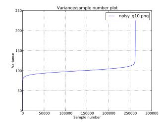
FIGURE 4. values of  $\mathbf{V}[\mathbf{I}Vn]$  depending on n using  $21 \times 21$  blocks without any filtering in the image of pure white Gaussian noise (figure 2, right). If the percentile is under the median one obtains an underestimated value; if it is above the median, an overestimation. The median is attained at position  $n = \frac{(N_x - w + 1)(N_y - w + 1)}{2} = \frac{(704 - 21 + 1)(469 - 21 + 1)}{2} = 153558.$
