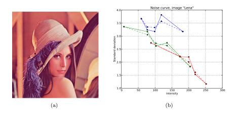
FIGURE 3. (a): test image *Lena* used to compare the noise curves with and without filtering; (b): noise curve for *Lena*. The non-filtered curve is drawn with solid lines and the filtered curve (five iterations) with dashed lines, using D = 7, p = 0.5%, w = 8 and 6 bins. Note that the peak in the blue channel is corrected after the filtering.
