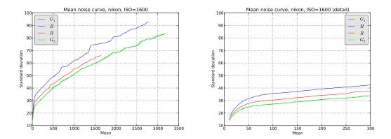
FIGURE 23. Mean noise curve for the Nikon camera with ISO 1600. Since this noise curve was obtained from raw images, it can be used as the ground-truth of the noise of the camera for that ISO. On the right, a detail of the curve at the darkest pixels.
