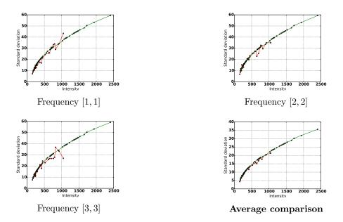
FIGURE 5. Comparison of the temporal (ground-truth, in green) and spatial STD (in red) for the Canon EOS 30D in raw images for ISO speed 1600 using blocks of  $4 \times 4$  DCT coefficients. The temporal and spatial STD match despite some oscillation in the spatial estimation. The curve at the bottom right is the comparison between the averaged mean temporal STDs and the averaged mean spatial STDs (along all frequencies except DC), showing that on average both estimations match accurately.
