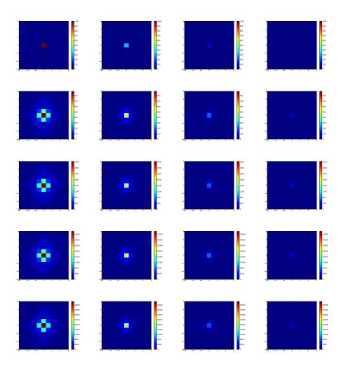
FIGURE 25. Autocorrelation functions for the Nikon camera, ISO 1600 and exposure time 1/250s. From up to bottom: results of the steps raw, demosaicing, white balance, gamma correction and JPEG correction. From left to right: first, second, third and fourth scales. Note that the scale of the color bar changes at each processing step.
