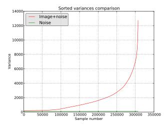
FIGURE 3. Values of  $\mathbf{V}[\mathbf{I}Vn]$  depending on n using  $21 \times 21$  blocks without any filtering in the noise-free test image *computer* after adding homoscedastic white Gaussian noise of  $\sigma = 10$  (red) and for pure homoscedastic white Gaussian noise of  $\sigma = 10$  image (green). Only a part of the values is shown. The estimation in the *computer* image is only reliable when the percentile of  $\mathbf{V}$  is small.
