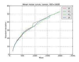
FIGURE 7. Ground-truth noise curve for the Canon EOS 30D camera, for ISO speed 1600.
