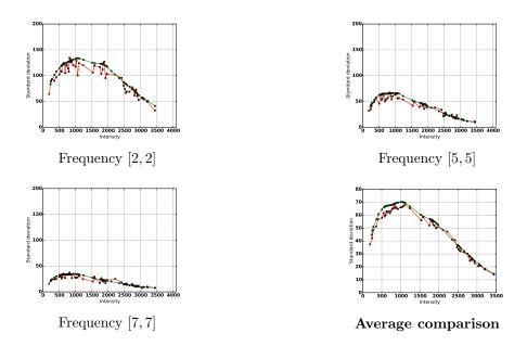
FIGURE 8. Comparison of the temporal (ground-truth, in green) and spatial STD (in red) for the Canon EOS 30D in JPEG-encoded images with quality factor Q = 92 for ISO speed 1600 using blocks of  $8 \times 8$  DCT coefficients. The curve at the bottom right is the comparison between the averaged temporal STDs and the averaged mean spatial STDs (along all frequencies except DC), showing that on average both estimations match.
