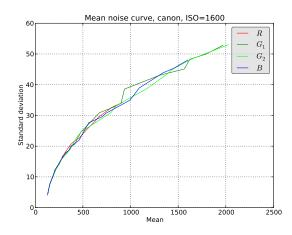
FIGURE 4. Ground truth of the Canon EOS 30D camera with ISO=1600.
