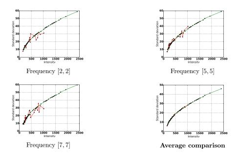
FIGURE 6. Comparison of the temporal (ground-truth, in green) and spatial STD (in red) for the Canon EOS 30D in raw images for ISO speed 1600 using blocks of  $8 \times 8$  DCT coefficients. The temporal and spatial STD match despite some oscillation in the spatial estimation. The curve at the bottom right is the comparison between the averaged mean temporal STDs and the averaged mean spatial STDs (along all frequencies except DC), showing that on average both estimations match accurately.
