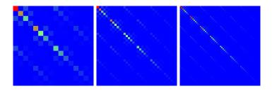
FIGURE 1. Visualization of the noise covariance matrices in DCT space after applying filter  $\mathbf{H}_1$  to illustrate that it is almost diagonal. From left to right, top to bottom patch size  $\kappa = 4, 6, 8$ .
