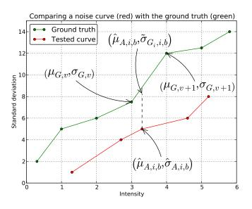
FIGURE 5. Checking a noise curve A (red) against the ground truth G (green), where *i* is the index of the image, *b* is the index of the bin,  $(\hat{\mu}_{A,i,b}, \hat{\sigma}_{A,i,b})$  are the control points of the noise curve A,  $(\mu_{G,v}, \sigma_{G,v})$  are the control points of G, and  $\tilde{\sigma}_{G_i,i,b}$  is the standard deviation value projected from A into G.
