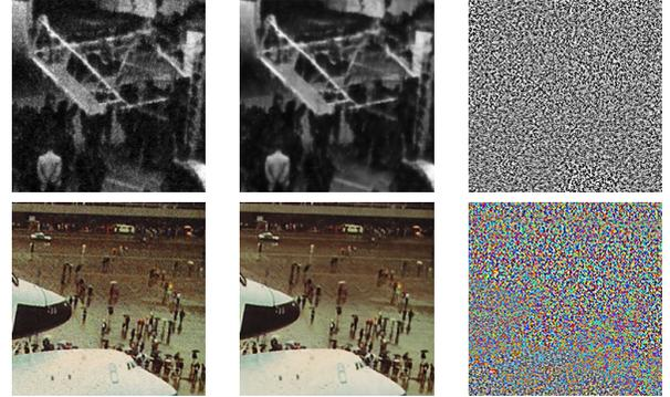
**Fig. 2.** Denoising results of real images with unknown noise model encoded with JPEG with unknown quality factor parameters. Left: detail of the noisy image. Middle: detail of the denoised image. Right: difference image (removed noise). The noise estimation method is validated, since the colored noise is removed (see the color spots in the difference image and its random geometry at zones with the same intensity) whereas signal detail is kept.
