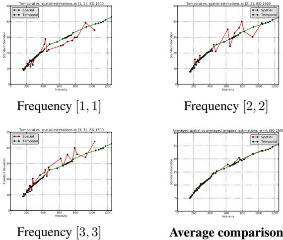
**Fig. 4.** Comparison of the temporal (GT, in green) and spatial STD (in red) for the Canon EOS 30D in raw images for ISO speed 1600 using blocks of  $4 \times 4$  DCT coefficients. The temporal and spatial STD match despite some oscillation in the spatial estimation. The curve at the bottom right is the comparison between the averaged mean temporal STDs and the averaged mean spatial STDs (along all frequencies except DC), showing that in average both estimations match accurately.
