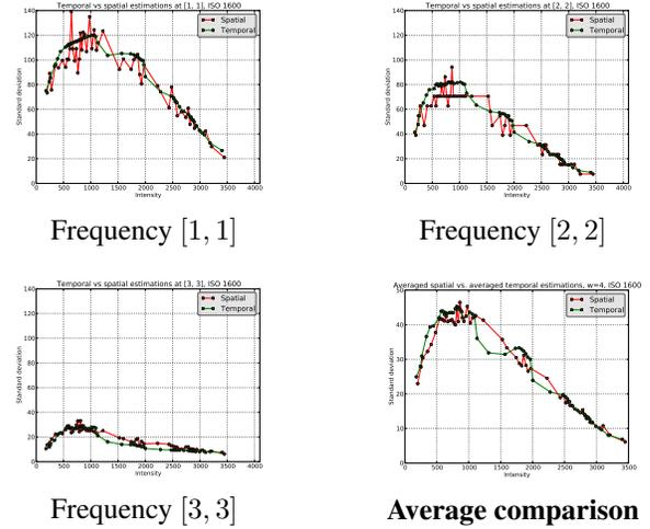
**Fig. 5.** Comparison of the temporal (GT, in green) and spatial STD (in red) for the Canon EOS 30D in JPEG-encoded images with quality factor  $Q = 92$  for ISO speed 1600 using blocks of  $4 \times 4$  DCT coefficients. The curve at the bottom right is the comparison between the averaged temporal STDs and the averaged mean spatial STDs (along all frequencies except DC), showing that in average both estimations match.
